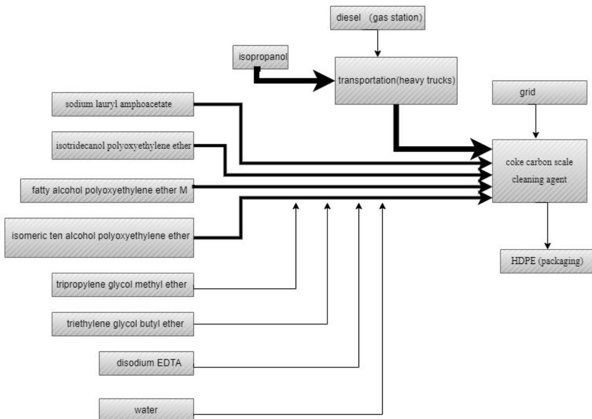
**Figure 1.** System boundary of the coke cleaning agent
