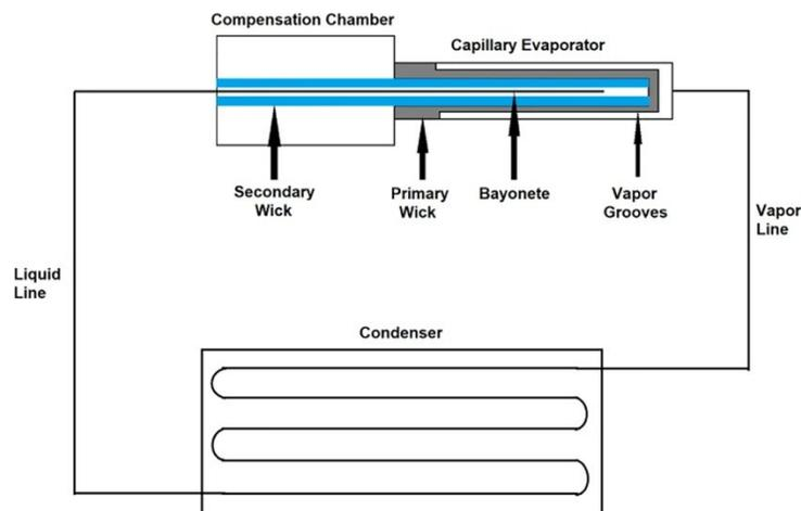
**Fig. 5.** Schematic Diagram of Loop Heat Pipe [32]
