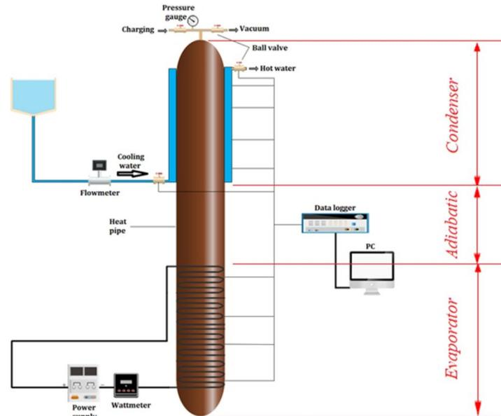
Fig. 8. Schematics of the heat pipe test rig [35]
