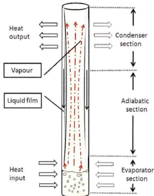
**Fig. 7.** Schematic Diagram of Gravity Heat Pipe
