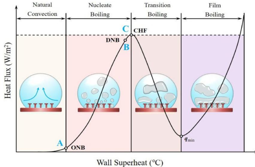
Fig. 4. Pool boiling curve [16]
