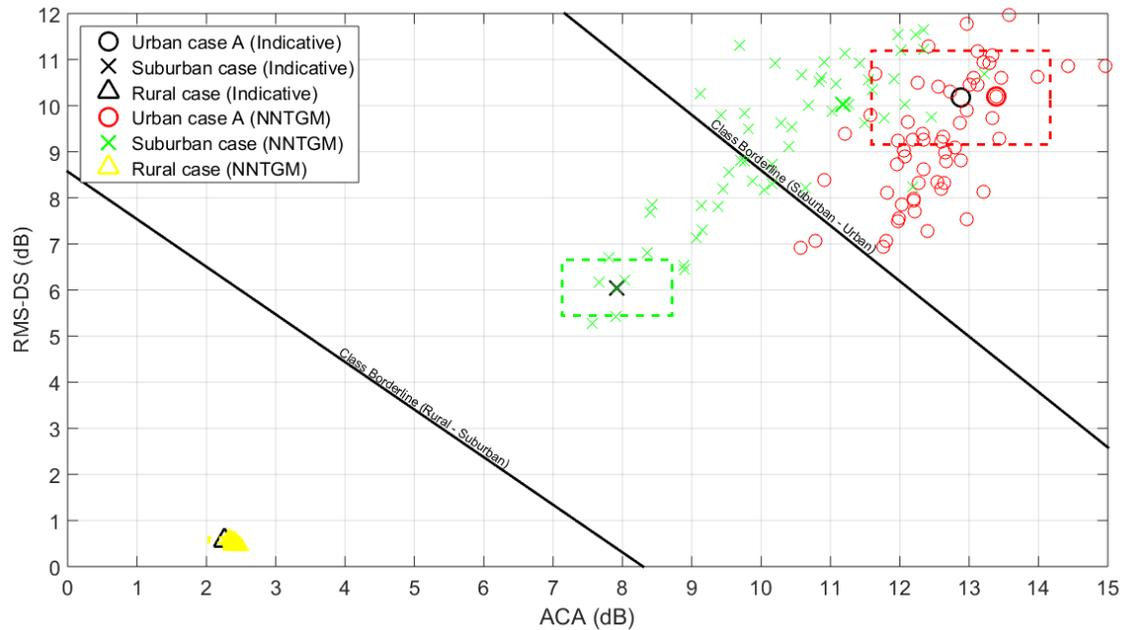
**Fig. 5.** OV LV BPL topology class map with NNTGM virtual topology footprints of the three indicative OV LV BPL topologies when the NNTGM default operation settings are applied but for training, validation and testing phase participation percentages being equal to 1%, 98% and 1%, respectively.
