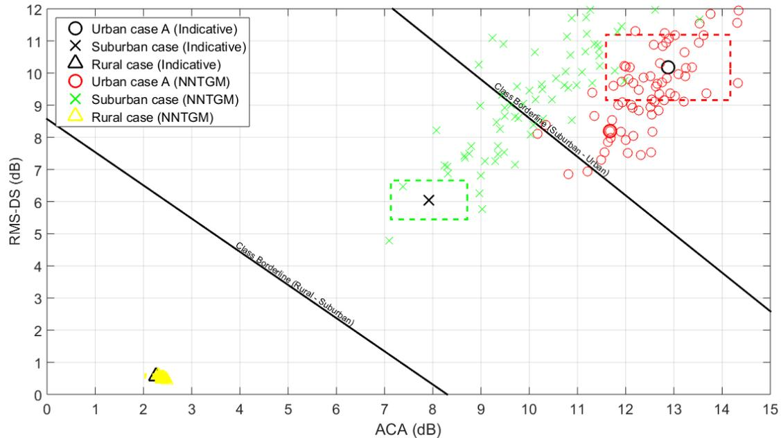
**Fig. 6.** OV LV BPL topology class map with NNTGM virtual topology footprints of the three indicative OV LV BPL topologies when the NNTGM default operation settings are applied but for training, validation and testing phase participation percentages being equal to 1%, 1% and 98%, respectively.
