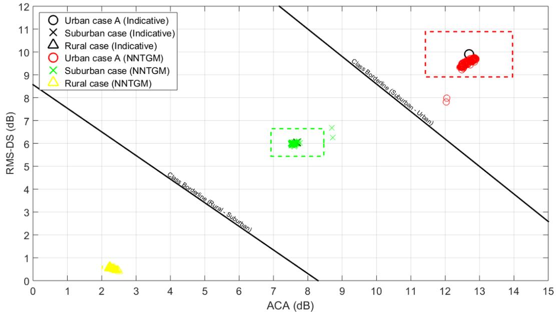
**Fig. 3.** OV LV BPL topology class map with NNTGM virtual topology footprints of the three indicative OV LV BPL topologies when the NNTGM default operation settings are applied but the flat-fading subchannel frequency spacing is equal to 2MHz.
