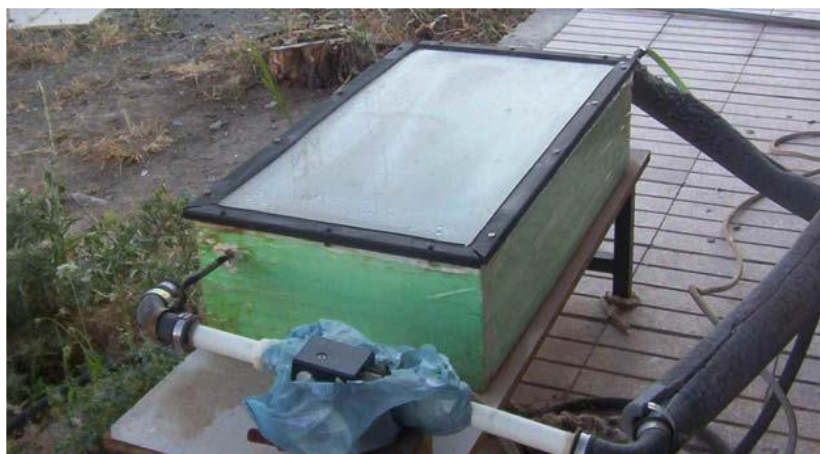
Figure 10. Experimental set up of the solar collector system using sodium carbonate decahydrate as PCM [43]
