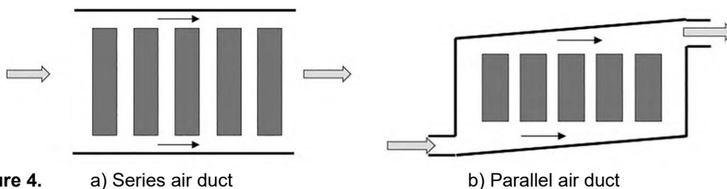
**Figure 4.** a) Series air duct
