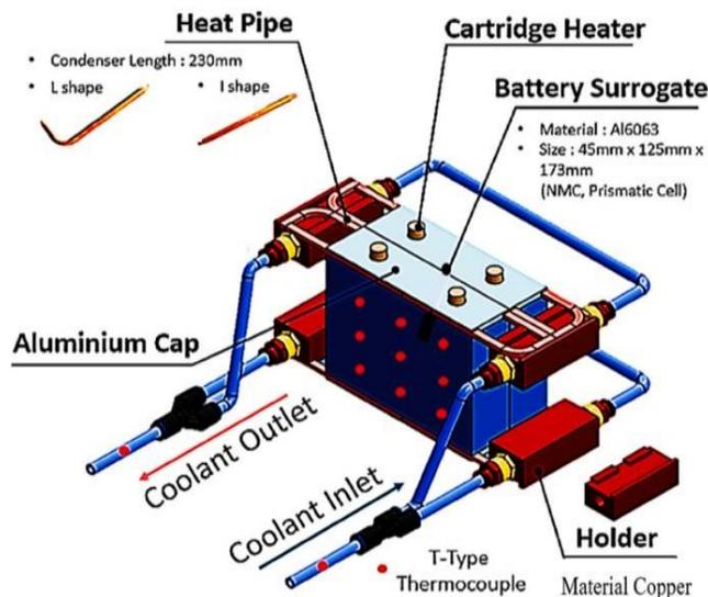
**Figure 8.** Battery BTMS based on L-shaped/I-shaped heat pipe [40].
