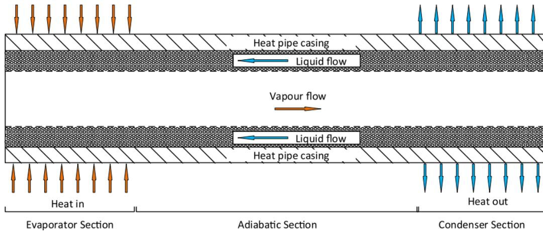
**Figure 7.** Cross-section of a conventional heat pipe[28].
