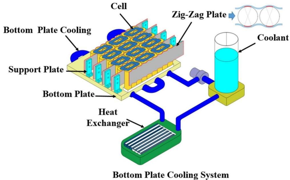
**Figure 5.** Bottom plate liquid cooling system [20].
