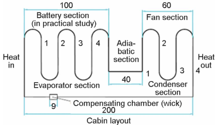
Figure 18. Line diagram of micro-heat pipe [43].
