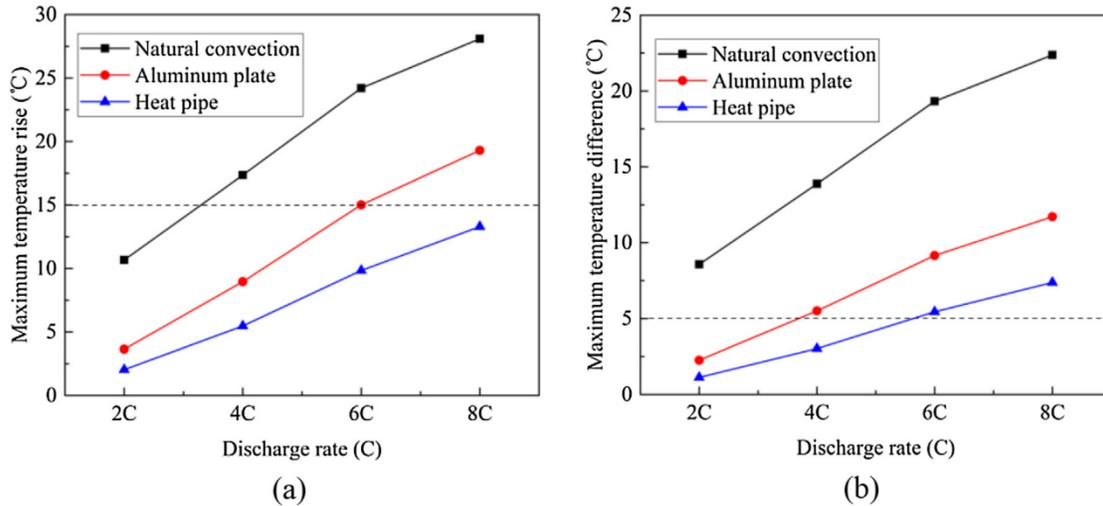
**Figure 9.** The maximum temperature rise and difference of the battery pack using different heat dissipation methods: (a) max temperature rise and (b) max temperature difference [30].
