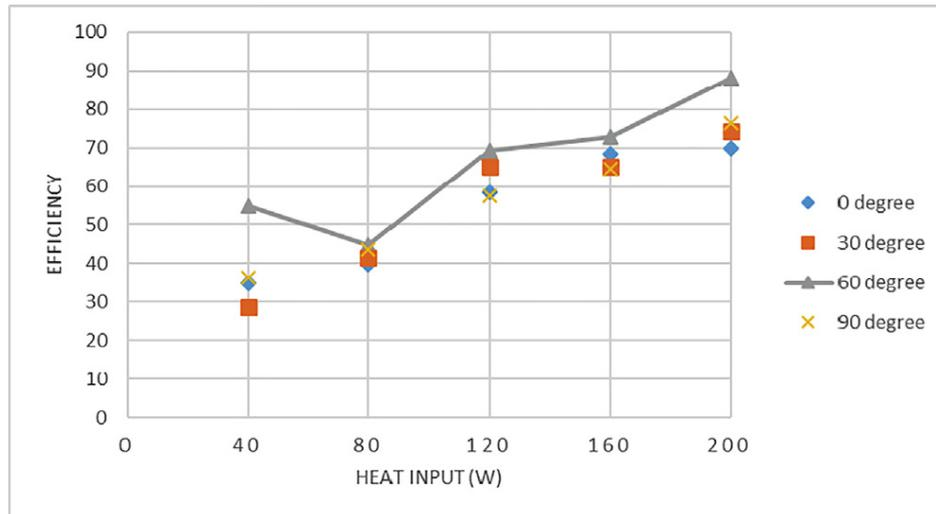
Figure 11. Efficiency of Heat Pipe with Nano Fluid [34].
