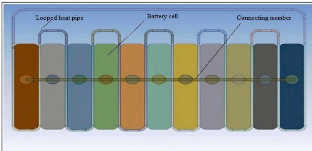
**Figure 17.** Arrangement of Li-ion battery cells with heat pipe[42].
